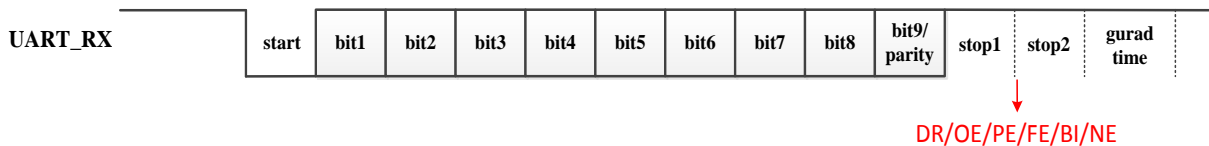
Figure 7-3 UART receiver flow
