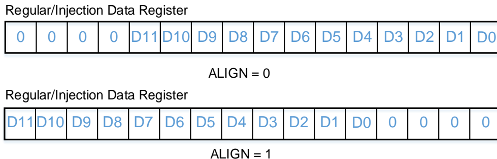
Figure 8-23 ADC data arrangement in data register
